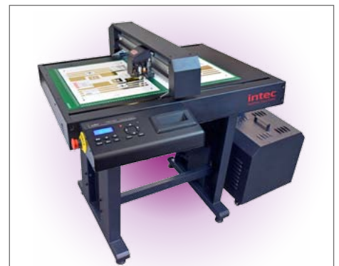
Barcode printed on both sides of sheet enables creasing from the rear as well as the front. This great feature is useful on particularly heavy or dense-fibred stock
