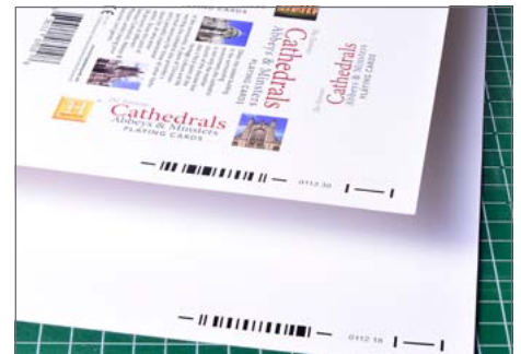
Barcode printed on both sides of sheet enables creasing from the rear as well as the front. This great feature is useful on particularly heavy or dense-fibred stock
