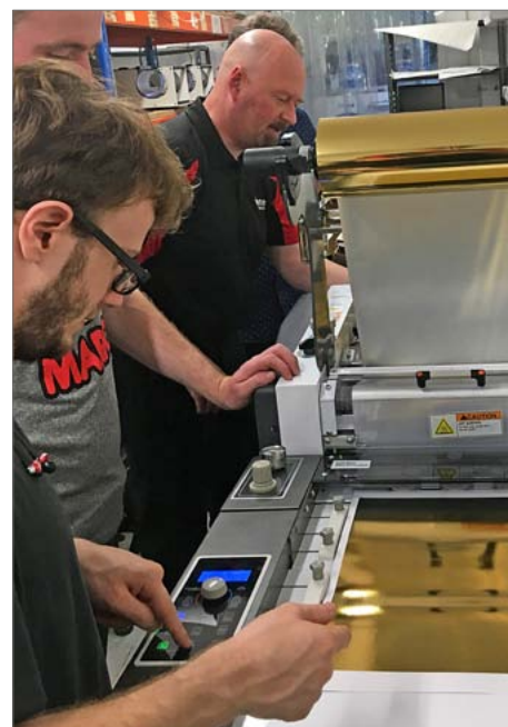
ColorFlare CF1200LX foiler / laminator being put through its paces on the installation day
