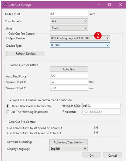
Switch off the cutter and wait 10 secs. Unplug the USB cable from your computer, and try a different port, then switch back on the ColorCut engine. Wait until the HOME screen is displayed on the LC600 LCD panel.
