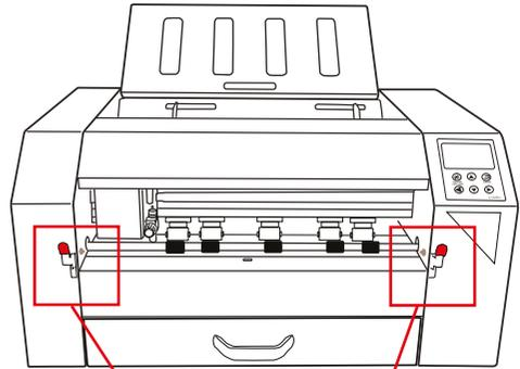
2. Open the Dual Drip Lever clamps to remove the Dual Grip Roller. In order to release the Dual Grip Lever, press in the ball catch ❷. (You may find it easier to use the end of a pen to do this).
