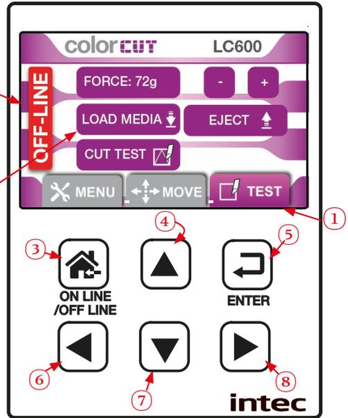
The TEST screen is very useful for checking your blade depth and the pressure/force used during cutting, prior to starting a job.
