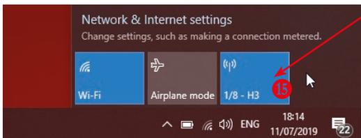
After enabling the mobile Hotspot, ensure you power ON the Intec LC600 cutter, and allow 30 secs - 2mins for it to connect to your HotSpot. Your Mobile HotSpot will show when the device is connected. **15**
