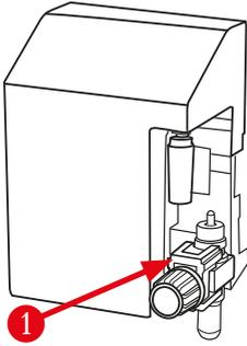
It contains a tool holder which enables you to easily and efficiently switch between different blade holders if required, or fit a pen for calibration purposes.
