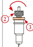
4. Replace the blade by following the steps above (or you can push the pin as you do with the standard method of replacing blades)
