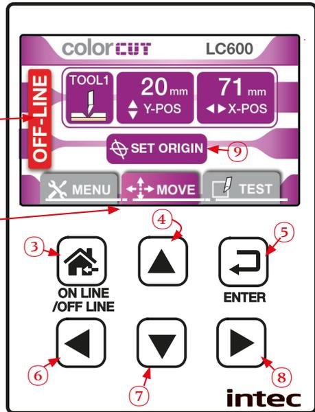
In the MOVE mode, the cutter status changes to [OFF Line] ② and will no longer receive new cutting files. When you have loading/ejecting media or moving the media/tool carriage press the [ **ON-LINE** ] ③ Key to return the cutter to the HOME screen, and change the LC600 cutter status back, to ONLINE.
