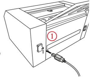
Securely plug the USB cable into the USB socket **1** on the rear panel and connect to your Windows PC.
