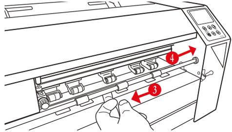
**5.** Replacing the Dual Grip Roller is the opposite procedure, diagonally fit the new bar towards the left and then down into position.
