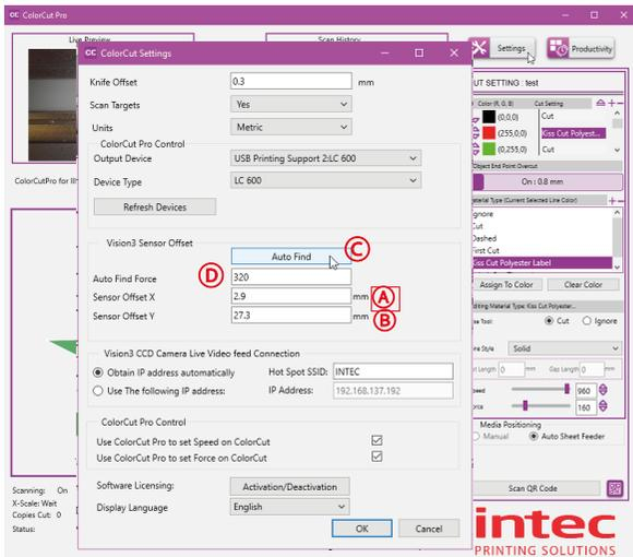
**7.** Click the [AutoFind] button, you will be asked to place media in the cutter, and click OK, then the Intec ColorCut LC600, will use the Pen Calibration Tool, to repeatedly draw a spiral pattern (E) to simulate a registration mark. it will then move the Vision3 sensor over to find the mark and automatically enter the values into your Sensor Offset X and Y settings. Once completed you will see a confirmation message.
