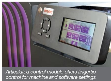
Articulated control module offers fingertip control for machine and software settings
