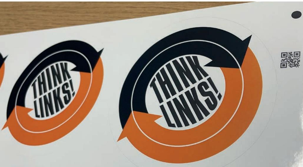
The SC5000 is also great for kiss cut labels. The cutter also has a facility for double depth cutting, where two blades are loaded, one to kiss cut and the other to cut through: Great for sticker packs.
