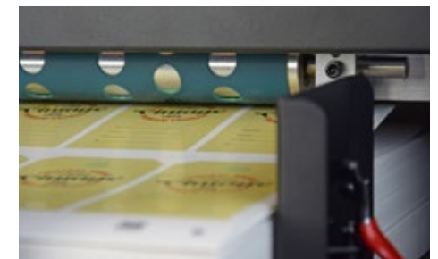
Continuous vacuum belt lifts and feeds sheets onto cutting bed ready for cutting
