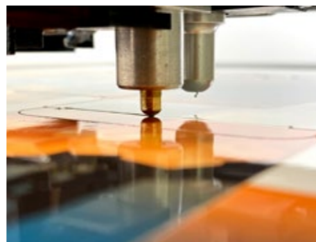
Cut and crease in one operation
