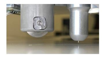
Tangential technology enables the FB9500 Pro-T to lift the tool away from the media, rotate it and place it back on the media. This type of creasing tool provides a smooth and more defined crease and is particularly good for thicker media.
