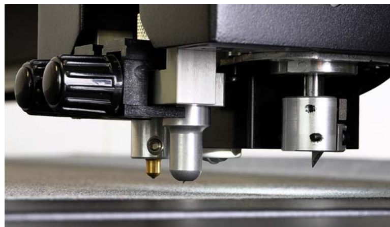
High force, rapid 4 tool head, includes 2 active tangential tools
