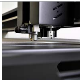
Quad tool head for rapid cut and crease capability
