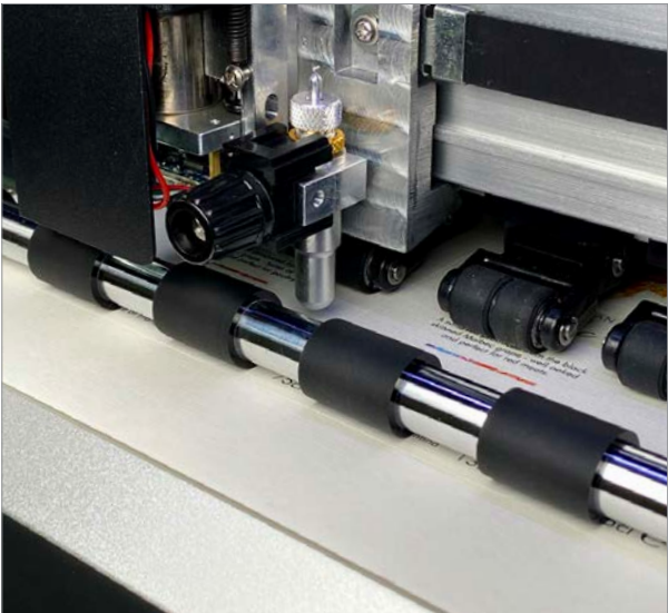
Blade holder offers blade changes dependent on media type
