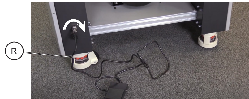
21. Plug the foot pedal cable [R] into the socket [S] on the front of the operator side panel. Ensure the plug aligns with the socket, then turn it clockwise to secure it.
