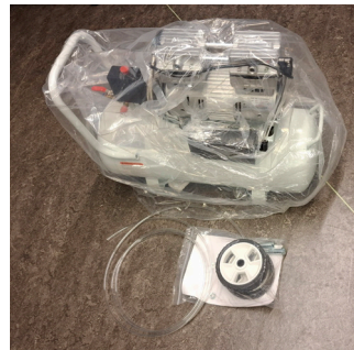
13. Open the back cover and cut security zip tie [P] on motor arm.
