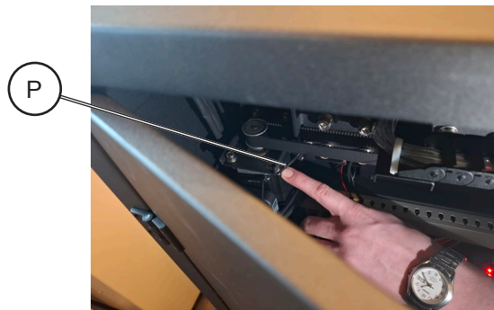
13. Open the back cover and cut security zip tie [P] on motor arm.
